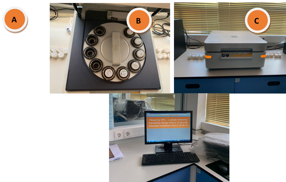
Gambar 2. XRF Spectrometry (PANalytical, Epsilon 3) ; (A) Sampel didalam XRF, (B) Uji XRF, (C) Analisis Hasil XRF (Dokumentasi Pribadi, 2021)
