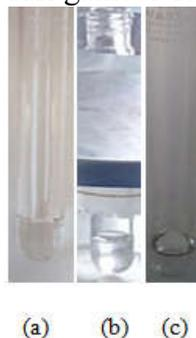
Gambar 1. Perbedaan (a) Mikroemulsi *water in oil* (b) Sol mikroemulsi *water in oil* (c) Gel mikroemulsi *water in oil*
