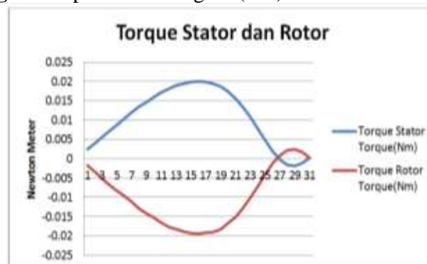
Figure 14. permanentmagnet (PM) : Ndfcb15° skewing
