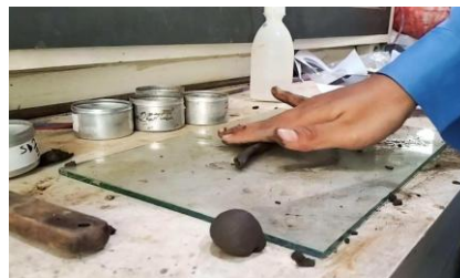
Gambar 2. Uji plastic limit (data hasil penelitian)
