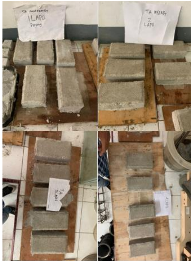
Gambar 4. Perawatan Benda Uji Paving Block
